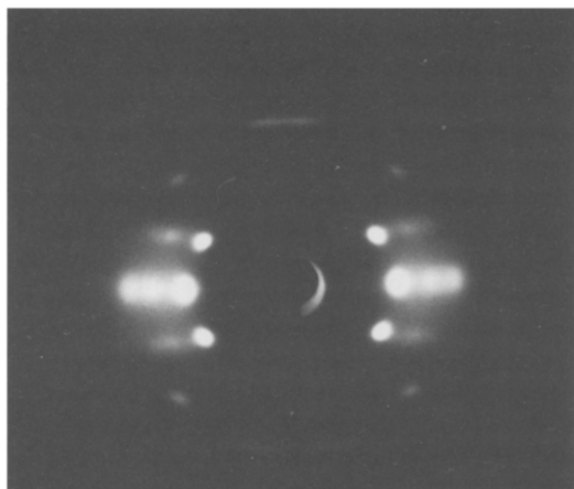
Figure 5 WAXS pattern of sample 3 (cold/hot zone drawn)
